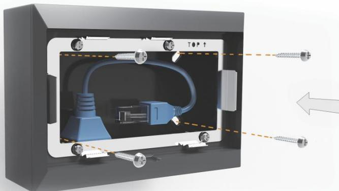
**Step 4:** connect the cable (blue) to the control panel
