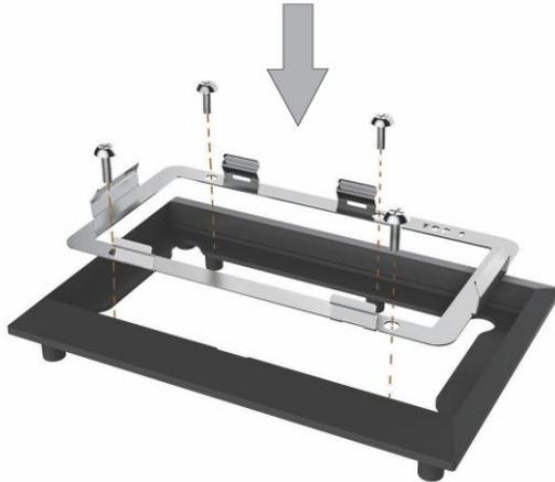
**Step 2:** tighten the top side to bottom side plastic part by the 4 screws
