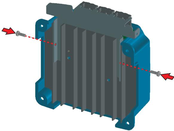
STEP 1: Mount the 'steel base' to the MPPT before installation to the wall.
