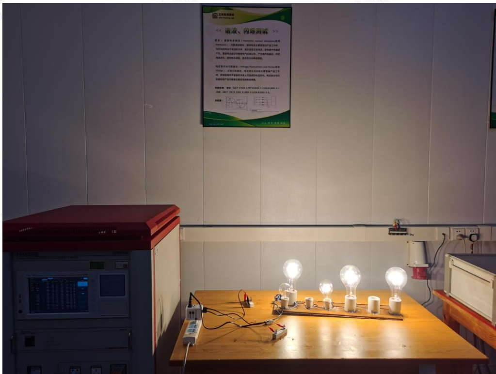
Test Setup Photo of Harmonic & Flicker Measurement
