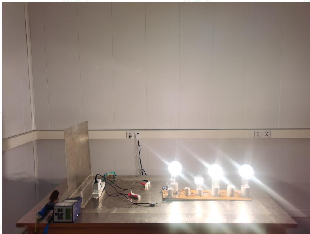
Test Setup Photo of Electrostatic Discharge Test
