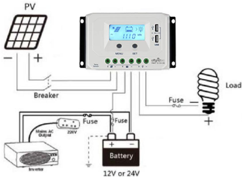
1. Connect components to the charge controller in the sequence as shown above. Pay much attention to “+” and “-”. Always connect the battery first in order to allow the controller to recognize the system voltage. Do not insert the fuse or turn on the breaker during installation. When disconnecting the system, the order will be reversed.
