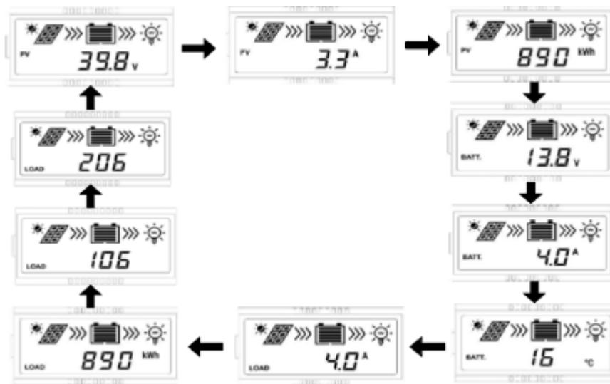
**Note:** When there is no operation the interface cycles automatically while the two displays shown below are left out.
