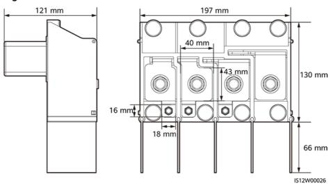
Figure 5-14 AC terminal block dimensions
