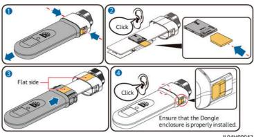
**Step 2** Secure the Smart Dongle.
