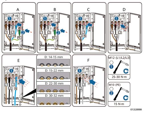
Figure 5-17 Cable connections
