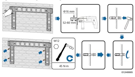
Figure 4-10 Installing the mounting bracket
