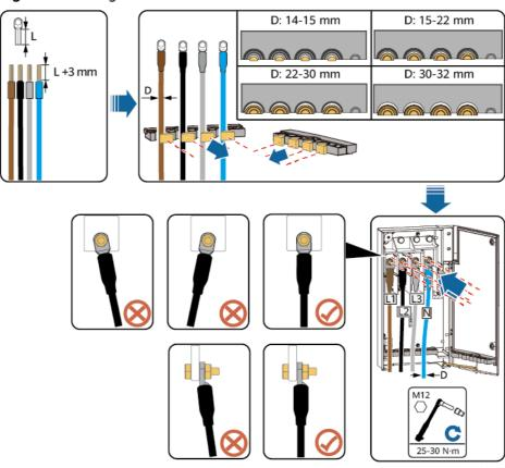
Figure 5-16 Single-core cable connections
