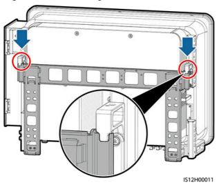
Figure 4-16 Mounting the solar inverter
