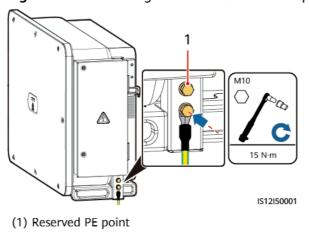
**Figure 5-6** Connecting the PE cable to the PE point (on the enclosure)
