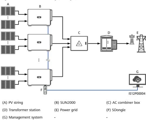
Figure 5-2 RS485 networking (SDongle)
