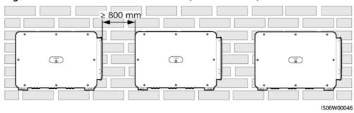
Figure 4-5 Triangle installation mode (recommended)
