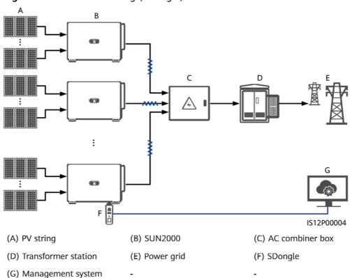
Figure 5-4 MBUS networking (SDongle)
