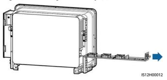
**Step 4** Remove cable ties from the faulty fan.
