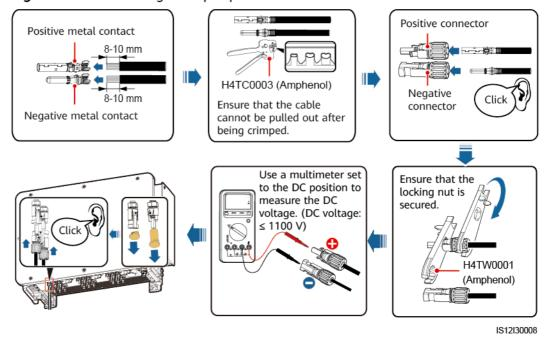
Figure 5-24 Connector connection
