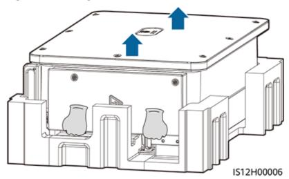
**Step 2** Lift the solar inverter and keep it upright.
