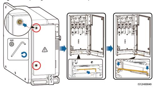
Figure 5-7 Opening the maintenance compartment door
