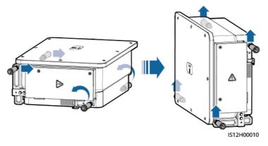
**Step 3** If the installation position is too high to install the solar inverter on the mounting bracket, run a rope that is strong enough to bear the solar inverter through the two lifting eyes, and hoist the solar inverter.
