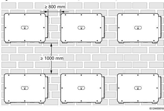
Figure 4-6 Stacked installation mode (not recommended)
