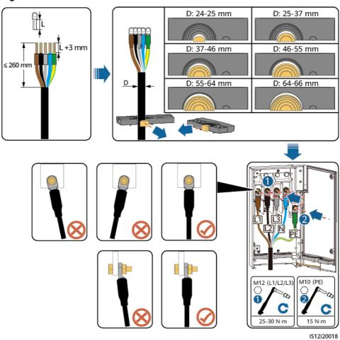
Figure 5-15 Multi-core cable connections
