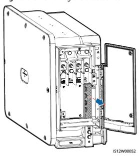
Figure 5-8 Removing the accessories
