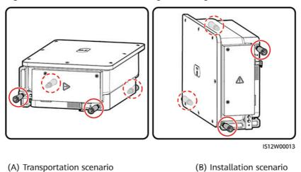
Figure 4-12 Lifting positions
