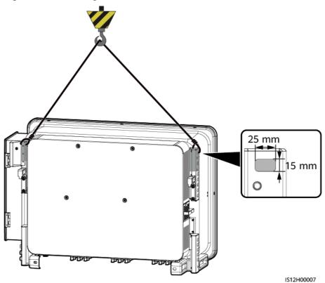
Figure 4-15 Hoisting the solar inverter
